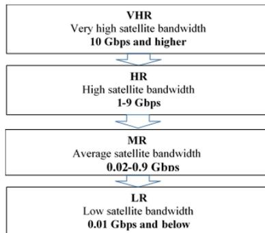
**Figure 4.** Bandwidth levels of communication satellites
