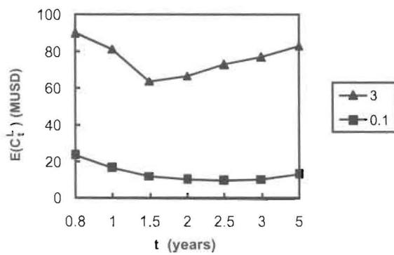
Figure 6. Expected life-cycle costs for Cuto Bridge. Optimal points are indicated for  $C_{St} = 3$  and 0.1 million USD (MUSD).
