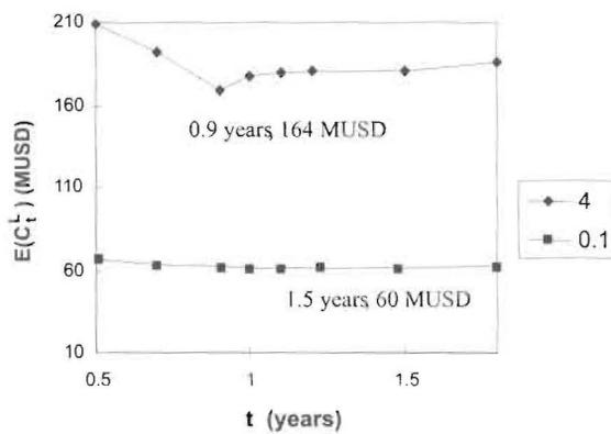
Figure 7. Expected life-cycle costs for Guadalupe Bridge. Optimal points are indicated for  $C_{St} = 4$  and 0.1 million USD (MUSD).
