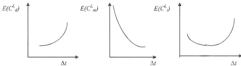
Figure 1. Conceptual maintenance cost functions.
