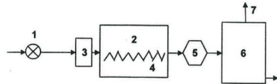
Figure 1. Modifiable extruder CZ 21314 U1. 1: high-pressure screw pump, 2: high-pressure reactor, 3: material heater, 4: internal screw for material transport, 5: expansion tourniquet, 6: expansion tank, 7: steam exhaust.
