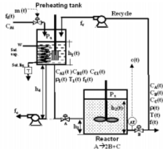
Figure 1. Process Diagram.
