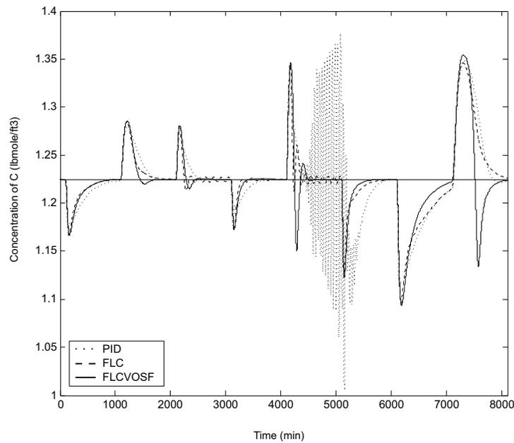
Figure 8. Process response to the steps in  $C_{Ai}$ .
