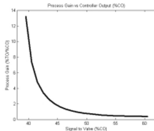
Figure 2. Process gain versus signal to valve.
