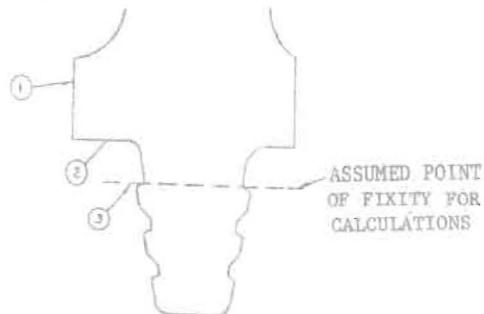
Figure 1 Assumed Point of Attachment of Beam for Analysis, From Jarret and Warner (25).
