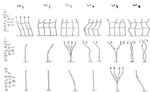
Figure 5 Relative Mode Shapes of a Four-Blade doubly-Laced Blade Group at 3600 rpm. From Deak and Baird, (100).
