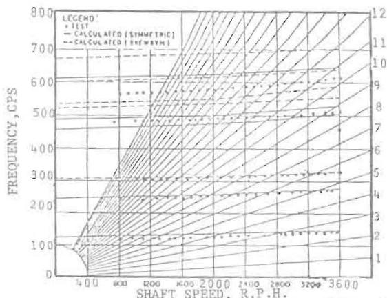
Figure 6 Campbell Diagram for Four-Blade Group with Two Tie-Wires, From Deak and Baird (100).
