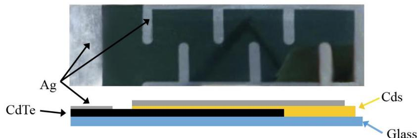
**Figure 4.** Details of the design of the p-CdTe / n-CdS cell. At the bottom, the experimental arrangement used in this work. In the upper part, photograph of the cell already made.
