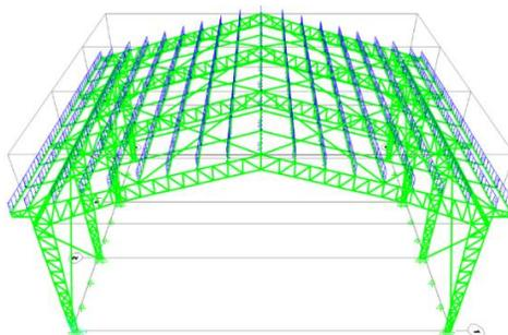
**Figure 2.** Live load and dead load of industrial buildings.
