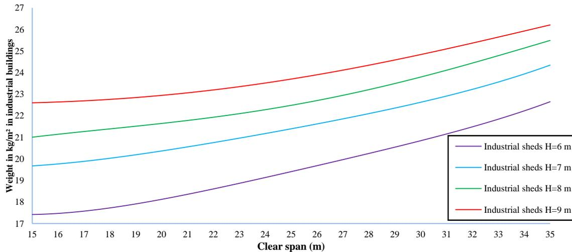
**Figure 5.** Interpolation curves (abacus) for industrial sheds with 5 m modulations.
