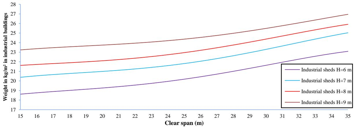
**Figure 6.** Interpolation curves (abacus) for industrial sheds with 6 m modulations.
