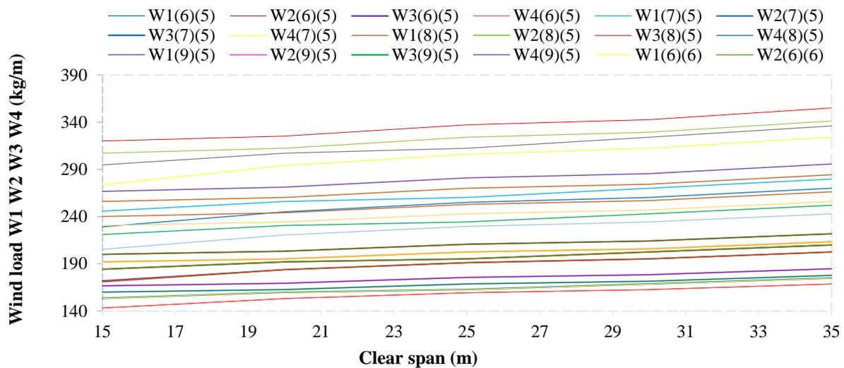
**Figure 4.** Summary of wind loads (W1, W2, W3 and W4) for industrial buildings with modulation between frames B = 5 and 6 m (windward).
