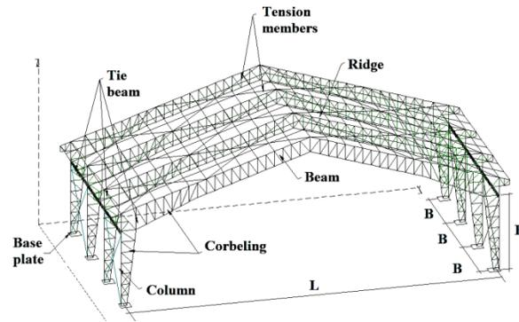
**Figure 1.** Geometry and variants of a metallic industrial building.
