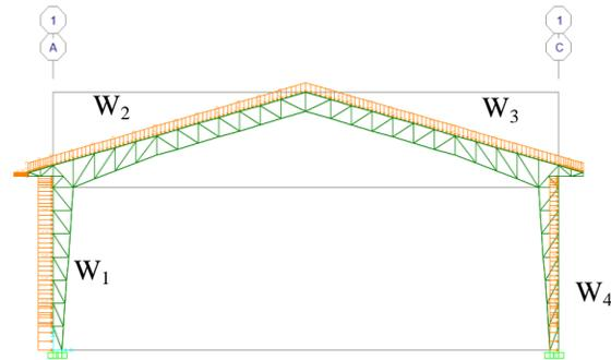
**Figure 3.** Wind load of industrial buildings. W1: windward column, W2: windward beam, W3: leeward beam, W4: leeward column.
