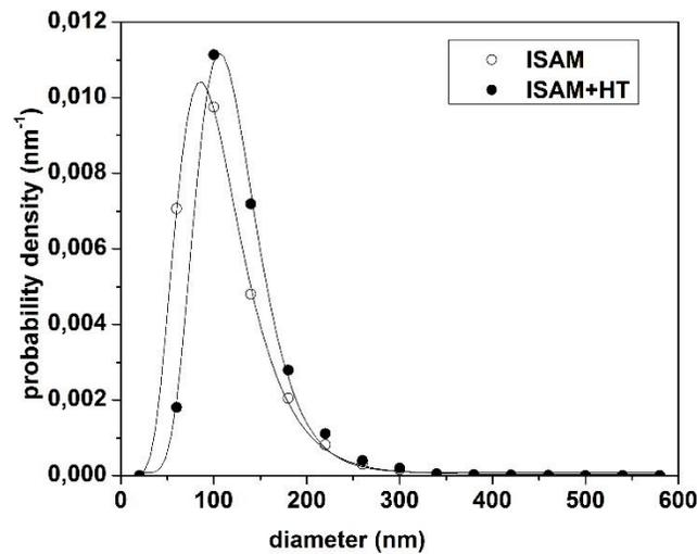
**Figure 4.** Experimental points and particle density curves of the ISAM (in-service aged material) and ISAM+HT (in-service aged material and subjected to heat treatment) conditions.
