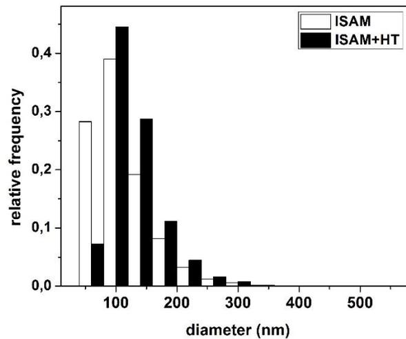
**Figure 3.** Relative frequency histograms of precipitate sizes for the ISAM (in-service aged material) and ISAM+HT (in-service aged material and subjected to heat treatment) conditions.
