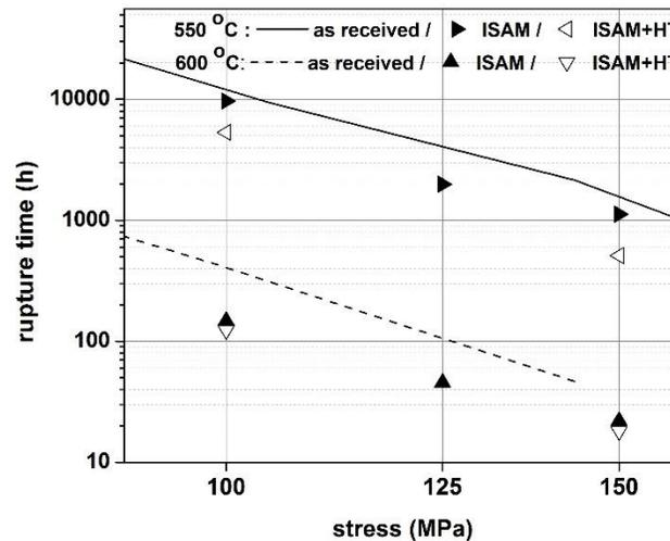
**Figure 6.** Creep rupture time from the experimental conditions ISAM (in-service aged material) and ISAM+HT (in-service aged material and subjected to heat treatment) and the as-received condition (Demirkol 1999).
