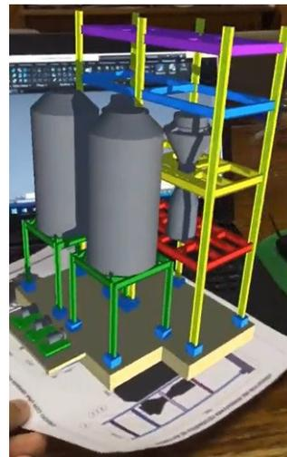
**Figure 3.** a) Mechanical structure drawing that serves as a marker. b) AR display through the Scope® app.
