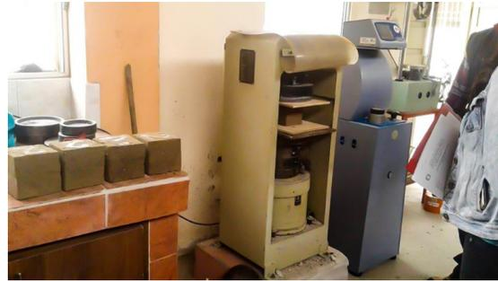
**Figure 1.** Standardized adobe samples for the test in the compression machine.
