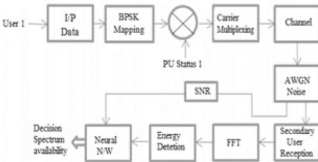
Figure(2): Flow mechanism of Neural Network based Spectrum sensing
