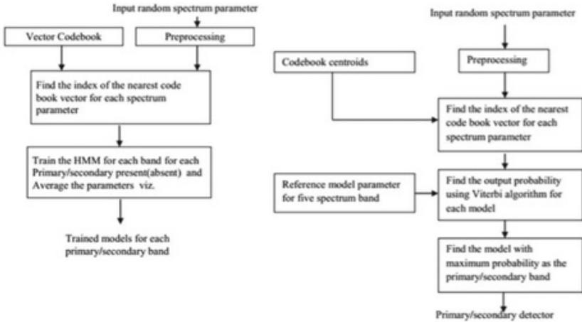
Figure(6):Block diagram of HMM training and recognition
