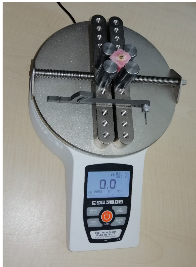
FIGURE 5. Performing the torque analysis with a digital torqmeter (Mark 10, NY, USA).
